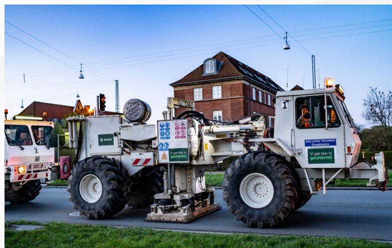
Four vibro-trucks drove through the streets of Aarhus in early May to map the subsurface.
